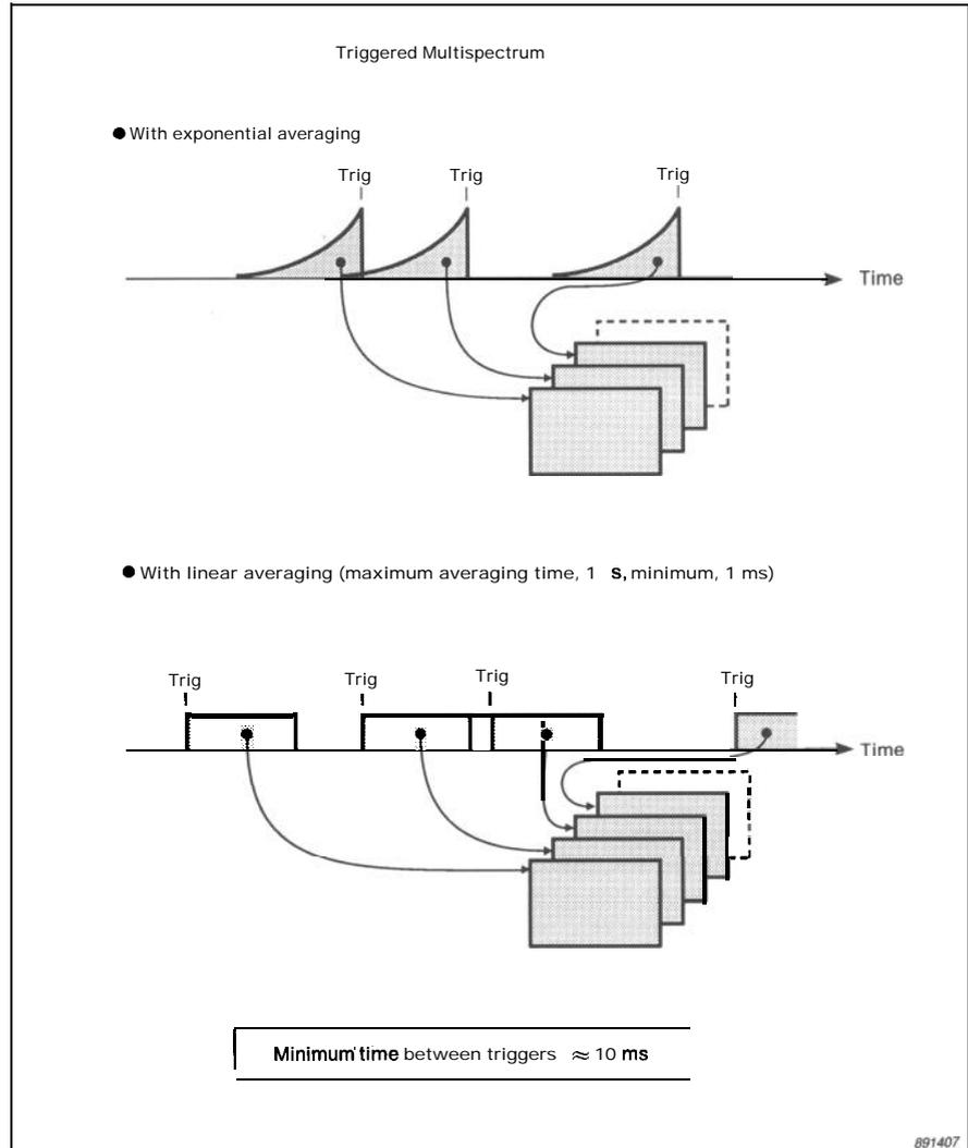
Fig. 8. Operation of the 2123/33 with triggered multispectrum
