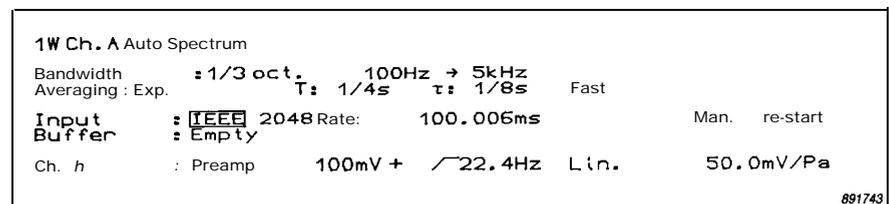
Fig. 10. Typical measurement set-up for spectrum history mode
